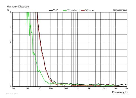
Measuring conditions, Harmonic Distortion Driver mounting: In sealed, heavily stuffed enclosure, internal volume 1.0 lit. Microphone distance: 0.5 m Input signal: Stepped sine wave, 2.0 VRMS (FR084WA01) / 2.83 VRMS (FR084WA02) Smoothing: 1/6 oct.
