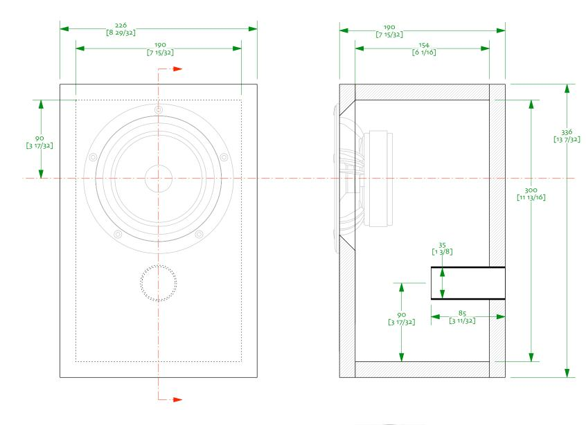
Notes: o/ designed for the Mark Audio Alpair 11ms – 8.5 litres 1/ drawn with 18mm material. Quality multi-ply recommended 2/ lag top, back, and one sidewall with 12-18mm cotton or wool felt or similar. Avoid acoustic foam 3/ bracing is optional but recommended 4/ don't forget to open up the back of the driver cut-out
