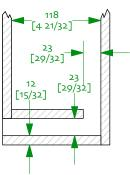
slot vent with 12mm box turned 90° so 110mm internal width, 118mm depth (for graham)
