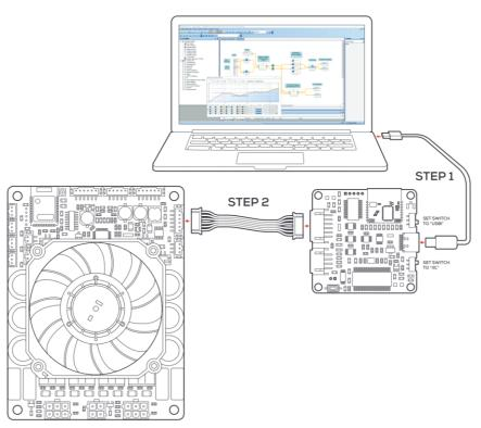
Pictured is a KABD-4100 amplifier connected to the KPX, which is connected to a Windows Laptop running the SigmaStudio software.
