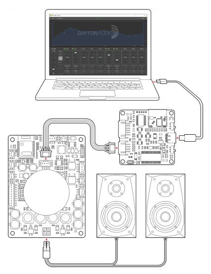
Pictured is a KAB-250v4 amplifier connected to the KPX programmer, which is connected to a Windows laptop running the KABX software.
