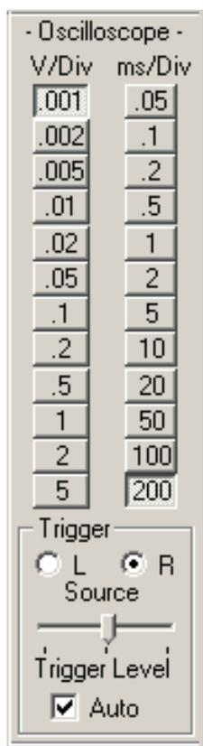
At the bottom is the trigger control group. A pair of buttons allow selection of either the left and right inputs for use as the scope's trigger signal. There is also a trigger level setting and an automatic triggering check box to switch the auto trigger on or off.
