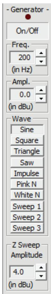
Below the Frequency field is the Amplitude field where you enter the desired signal level in dBu. Note that 0 dBu is 0.7746 Vrms. The up/down buttons allow the amplitude to be stepped up or down in steps of various sizes. Normally the amplitude is stepped in 1 dB increments. If the shift key is depressed the step size is increased to 10 dB. When the Ctrl key is held down the step size is reduced to 0.1 dB.
