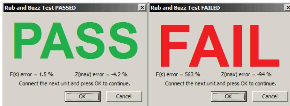
4. Connect the next unit under test and press “OK” to test the unit. For each unit tested the operator only needs to connect the unit and press ENTER (or click OK). The test procedure “loop” can be interrupted at any time by clicking the “Cancel” button. Resume testing using the current reference impedance by opening the Rub and Buzz setup dialog and clicking the “Resume Testing” button.
