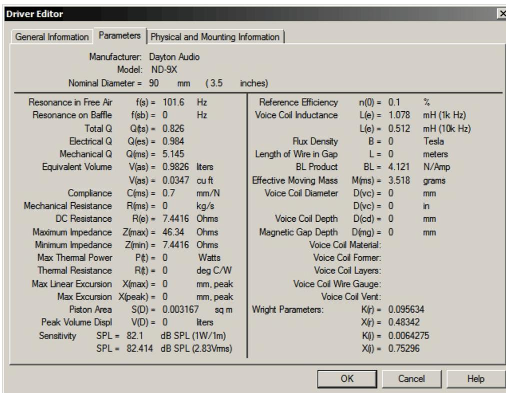
Note that several of the parameters are only seen here at the Driver Editor and are not displayed back at the main window. The parameters not displayed at the main window include: C(ms), Z(max), Z(min), S(D), n(0) and BL.
