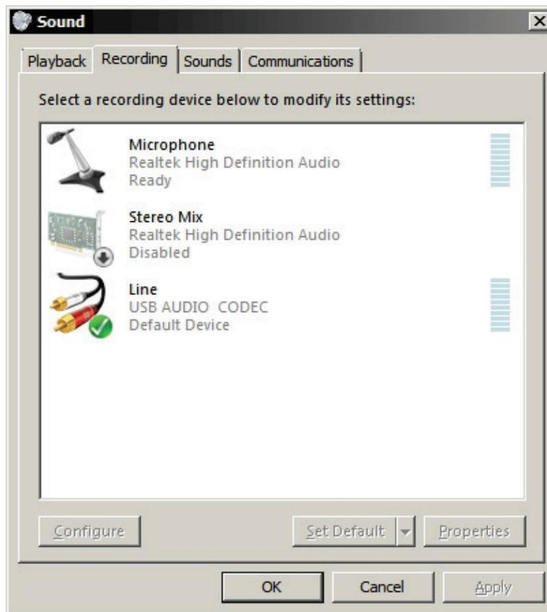
Next, double-click on the Line device "USB AUDIO CODEC" to open the Properties window seen below.
