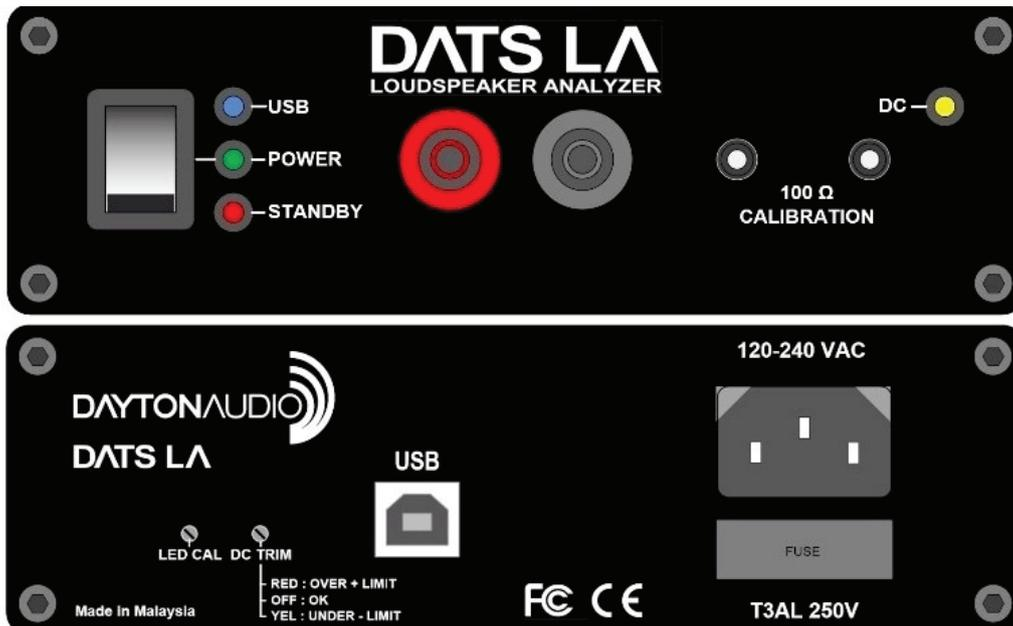
DATS LA introduces an audio interface unit with integrated calibration reference and front panel calibration terminals. The rugged aluminum module, powered by the USB port, comes with a detachable USB cable and test leads. The system operates with default Windows settings, requiring no adjustments. To ensure accuracy, the internal calibration resistor has a tolerance of  $\pm 0.1\%$ , achieving measurement accuracy better than  $\pm 0.5\%$  in the critical range between 1 Ohm and 1k Ohms.
