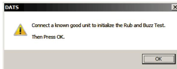
2. Connect a reference (known good) driver and click “OK” (or press ENTER at the keyboard). The reference unit is measured and its impedance is stored in memory 1. The dialog below appears.
