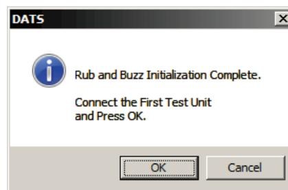
3. Connect the first unit to be tested and click “OK” (or press ENTER at the keyboard). The unit is tested and its impedance is stored in memory location 2. Either the PASS or the FAIL dialog will appear to indicate the test result as shown below.
